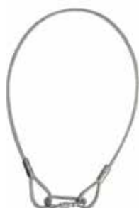
Safety Chain cod. 904PR TECHNICAL DATA Length: 75 cm Certified: BGV-C1 Ø: 6 mm; Incl.: Undetachable Carabine hook Finish: galvanized SWL: 80 Kg Safetyfactor: 5:1 Number of strands x number of wires: 6x19+TK Tensile grade: 1770N/mm2
