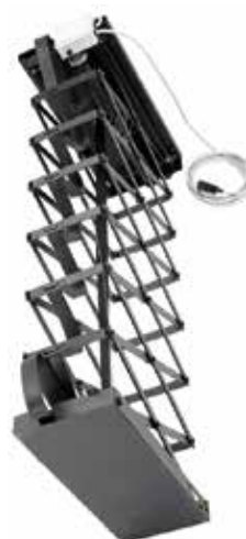
Elevator cod. AC343 TECHNICAL DATA Power supply 110/230Vac 50/60Hz. Power consumption: 250W Motor type: Tubolar 110/230V Housing: Iron Height Max 2700mm Max Load: 80kg Working position: Vertical CONTROL by Remote control Available with DMX cable Available with Audio cable SIZE: L710, W340, H260 Weight 53Kg
