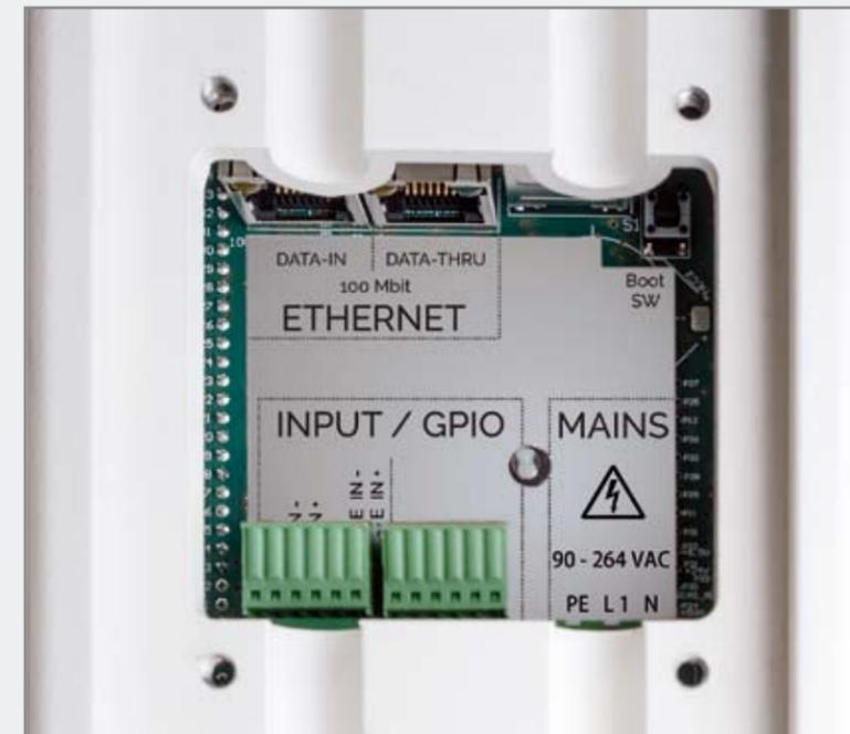
Cabling is done invisible, all connectors are hidden in a closed input board, and cables run in cable ducts. Thanks to the network-switch provided in every ALX connections from one to the next speaker can be done.
